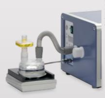
PWG-33BT provides full BTPS simulation for all types of exhaled curves
